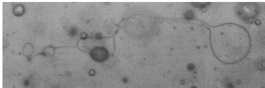
Fig. 9. Image of a breaking drop of silicone oil with \eta_D = 500 mPas, stabilized by 1 wt% Brij 58. The image is taken by a high-speed video camera (model PCO.1200hs, Samwoo Scientific Co., 700 frames/s) in a homogenizer equipped with optical window, which allows optical observation of the drops just after the narrow slit of the processing element.
