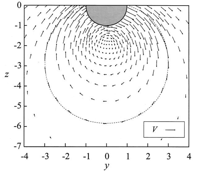
FIG. 9. Velocity field for a particle on a very viscous interface ( $E=30$ ). Input parameters are  $\eta_\alpha/\eta_\beta=1$ ,  $K=0$ ,  $R/a=3$ ,  $\bar{d}=0$ . The velocity field is shown in toroidal coordinates lattice presentation. The dotted line shows the position of the spherical interface.
