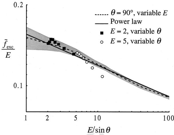
FIG. 6. Scaled excess friction  $\bar{f}_{\text{exc}}/E$  versus  $E/\sin\theta$  for a flat infinite membrane. See text and figure insert for definition of symbols. The gray band represents the estimated uncertainty of the computed values of  $\bar{f}_{\text{exc}}/E$ . As the relative uncertainty of  $\bar{f}$  is about constant, that of  $\bar{f}_{\text{exc}}/E$  diverges when  $\bar{f} \rightarrow 1$ , i.e., when  $E \rightarrow 0$ .
