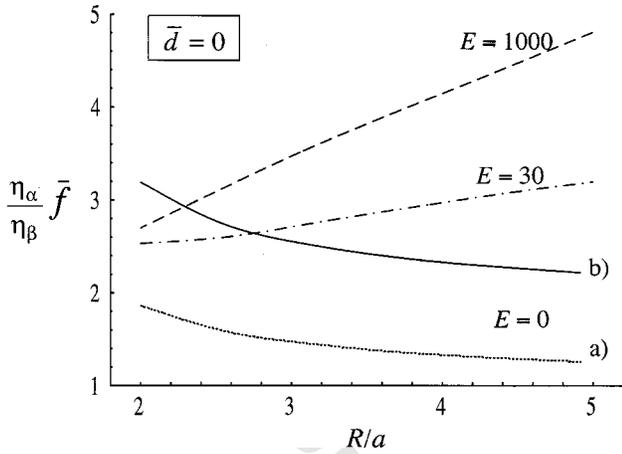
FIG. 8. Friction coefficient scaled to Stokes resistance for phase  $\beta$ .  $K=0$ ,  $\bar{d}=0$ . The two upper curves present results for high shear surface viscosity ( $E=30$  and  $E=1000$ ) and a viscosity ratio  $\eta_\alpha/\eta_\beta=1$ . The dotted line, curve (a), corresponds to a nonviscous surface,  $E=0$  and  $\eta_\alpha/\eta_\beta=1$ , while the solid line, curve (b), is calculated for  $E=0$  and  $\eta_\alpha/\eta_\beta=1.5$ .
