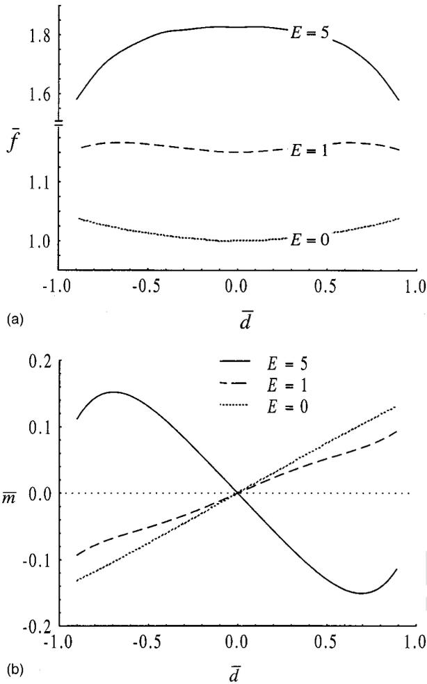
FIG. 5. Reduced friction (a) and torque (b) of a spherical particle across a flat interface  $K=0$  and  $\eta_\alpha/\eta_\beta=1$ . The dotted line corresponds to a nonviscous interface,  $E=0$ ; the broken and solid lines to  $E=1$  and  $E=5$ , respectively.
