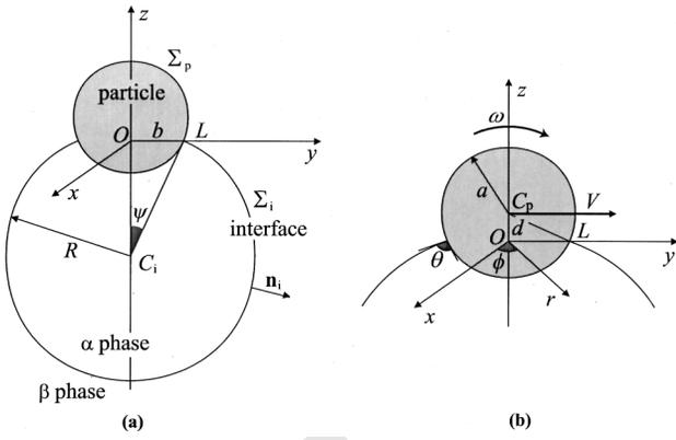
FIG. 1. (a) The problem: a particle of radius  $a$  across a spherical interface of radius  $R$  separating two fluid phases,  $\alpha$  and  $\beta$ ; (b) detail of the VDB-particle complex; see text for symbol definitions.
