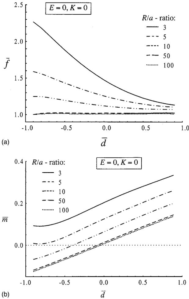
FIG. 4. Size ratio effect for a nonviscous interface ( $E=0, K=0$ ). Dimensionless drag coefficient  $\bar{f}$  (a) and torque coefficient  $\bar{m}$  (b), as a function of penetration depth,  $\bar{d}$ , for different size ratios,  $R/a$  (see the insert),  $\eta_\alpha/\eta_\beta=1$ .
