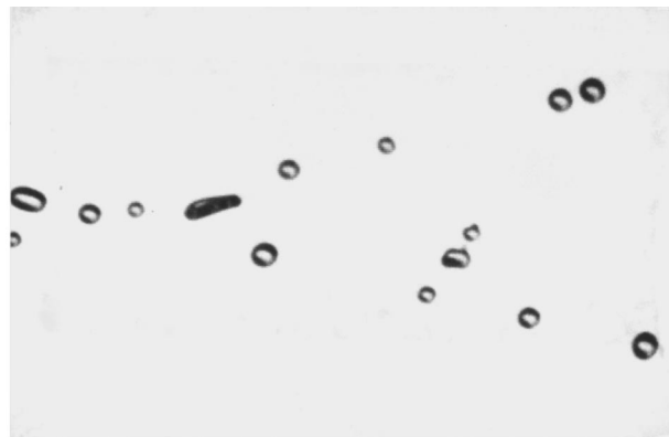
FIG. 8. Photograph of collisional interactions between two polydisperse drop streams with a larger magnification. This picture shows only a few drops close to the intersection point of the drop streams. Large merged drops can be seen. The photograph shows a section of the flow with a total length in the x direction of 5 mm.
