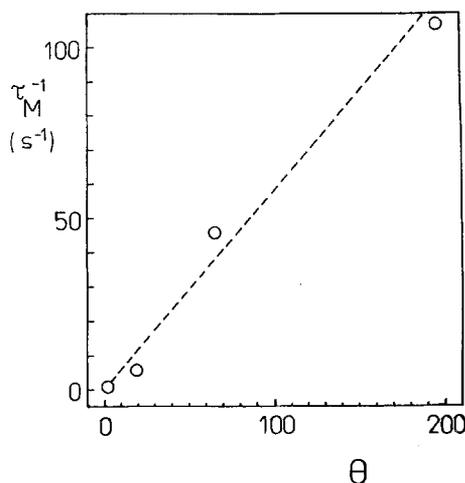
Fig. 3 Concentration dependence of the reverse relaxation time of micellization  $\tau_M^{-1}$  of Veranol H10 solutions computed from the data measured by the MBP-method at 25 °C [1] ( $\tau_D = 14.66 \text{ s}$ ). Dashed line is drawn as a guide for the eye
