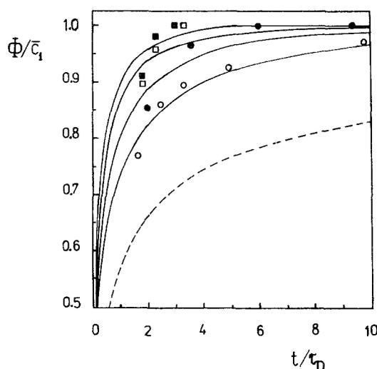
**Fig. 1** Subsurface concentration  $\Phi(t)$  of micellar SDS solutions with different surfactant concentration in mol/cm<sup>3</sup>:  $1.2 \times 10^{-5}$  (○);  $1.6 \times 10^{-5}$  (●);  $2.4 \times 10^{-5}$  (□);  $3.2 \times 10^{-5}$  (■). Data are measured by the MBP-method at 25°C [1]. The solid lines are drawn by Eq. (4.1), while the dashed line corresponds to the case below CMC [2] ( $\tau_D = 8.1 \times 10^{-3}$  s)
