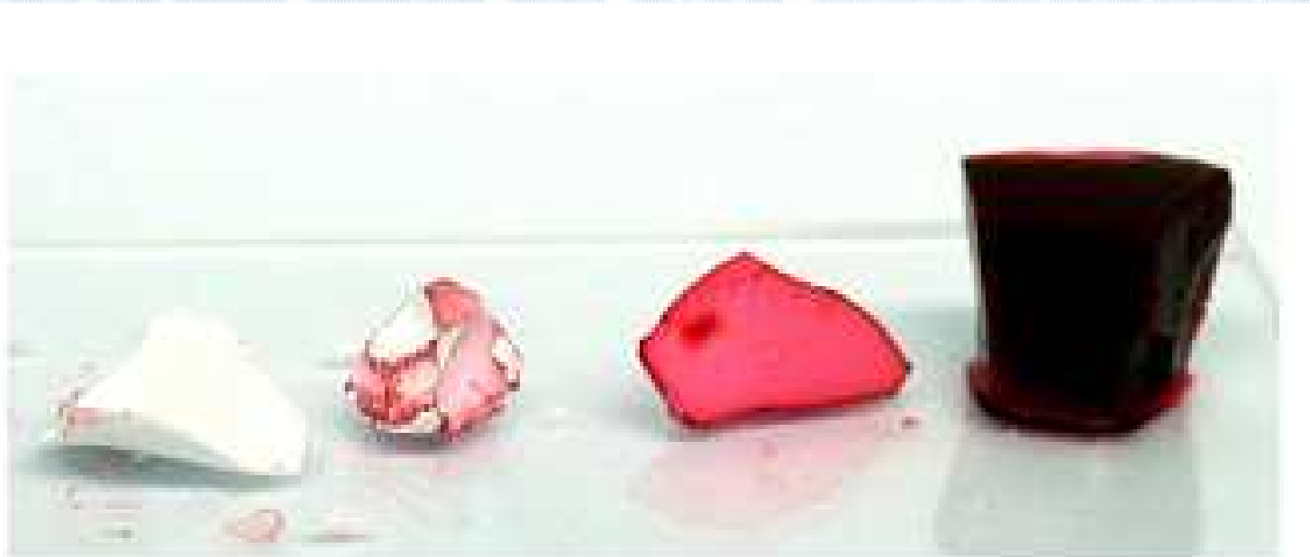
Fig. 6. Bulk sol-gel foams after immersion in a water: SDS mixture with red dye added. Samples from left (1) sample heated to 300 °C, no SDS; (2) sample heated to 300 °C, 0.08 M SDS; (3) sample unheated, 0.08 M SDS; (4) sample heated to 400 °C, 0.08 M SDS.
